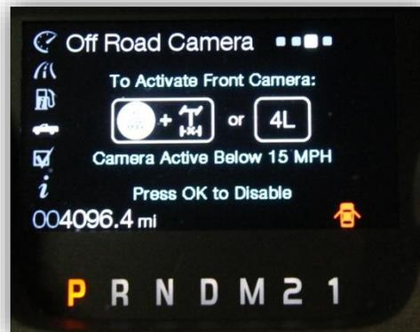
4. The front camera will display on the screen (the active steering lines will not be displayed), the cluster will display 'Press OK to disable'
