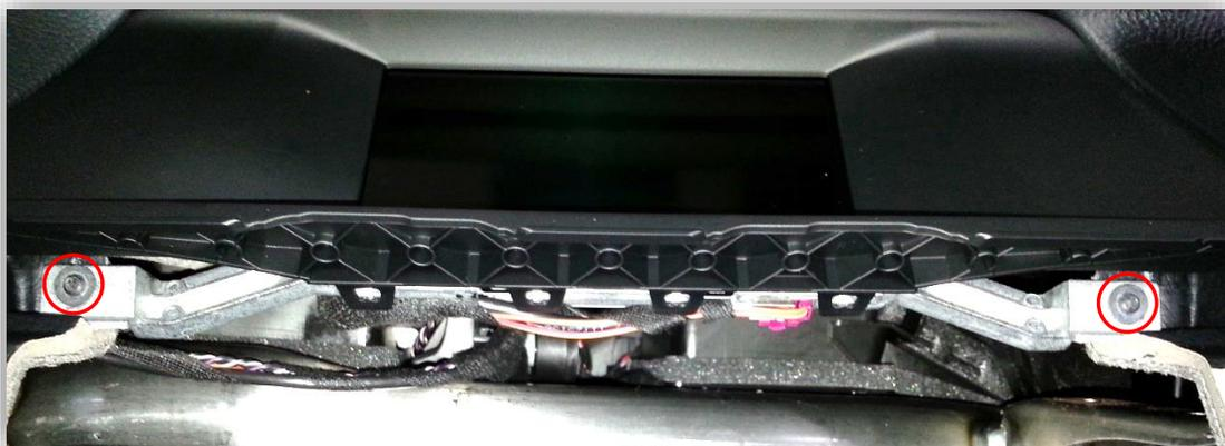
8. Remove the factory monitor, disconnect the LVDS video cable and remove it out of the dashboard. **This (factory) LVDS cable will connect between the radio and the BMW12 interface (LCD-IN).** Gather the LVDS video cable provided with the BMW12 kit. This LVDS cable will connect between the BMW12 interface and the factory LCD screen (LCD OUT). Use the labeled ports on the BMW12 interface to plug the cables in properly. These connectors are keyed and will only insert in one direction.
