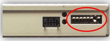
**\*Note: after adjusting Dip Switches, you must disconnect and reconnect power to the interface or the change will not be implemented.**
