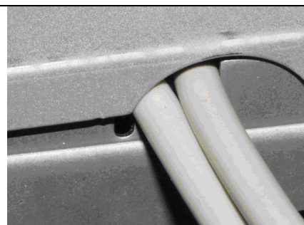
6. Route cable thru the small opening as depicted.
