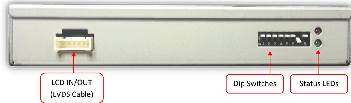
Dip Switch Settings\* Configure prior to installation
