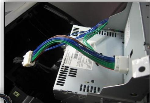
5. You are now left with a 5-pin **OEM IN** plug and an 8-pin **RGB OUT** plug. Connect these (2x) plugs to the ports labeled **OEM in** and **RGB OUT** on the FX KIT Interface:
