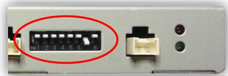
**\*Note: after adjusting Dip Switches, you must disconnect and reconnect power to the interface or the change will not be implemented.**
