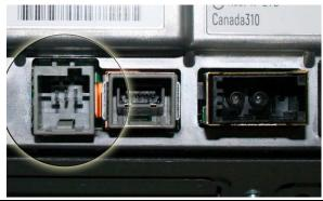
With the grey 6 pin connector locking tab facing upwards, the far right top and bottom slots are for the video input. The center top and bottom slots are the RVC video input. On both inputs the top is + and the bottom is negative.
