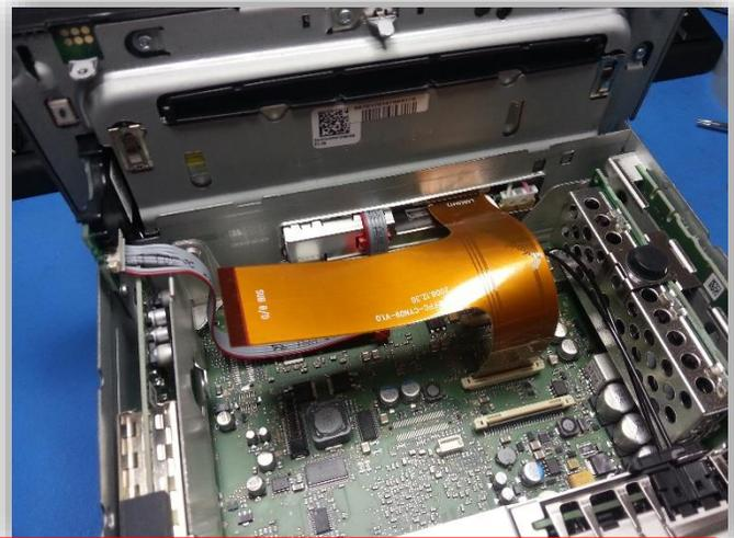
**\*Note: The proper direction and orientation of the cable is when the white font 'LCD(OUT), SUB B/D, LCD(IN)' is facing up or towards you (so that you can see it).**
