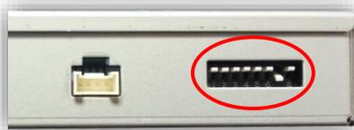
***\*Note: Disconnect power to the interface before adjusting dip switches or the change will not be implemented.***
