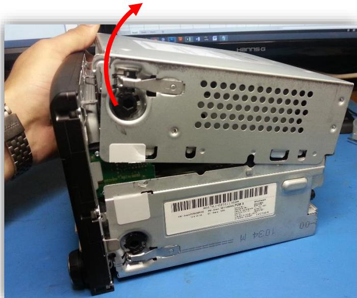
6. With a small flathead or a fingernail, carefully pry up the FFC cable connector that connects the disc drive ribbon. Set the disc drive aside.
