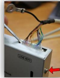
21. Connect the **AV Input** cable to the port on the RGB PCM3.0 interface labeled '**AV IN/OUT**'. If you're only connecting a reverse camera (and no other inputs), the signal input from the camera must connect to the RCA labeled '**R-CAM**'. Refer to the dip-switch settings chart to skip/enable AV sources upon toggle switch presses (optional. Page 2).
