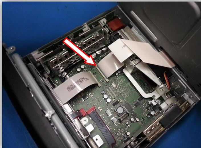
7. The ribbon indicated by the arrow will be replaced with the provided **Ribbon T-Cable**.
