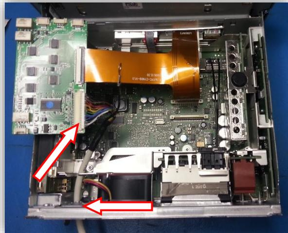
13. Ground the shield cable (with connected terminal) to the Torx screw on the radio as shown:
