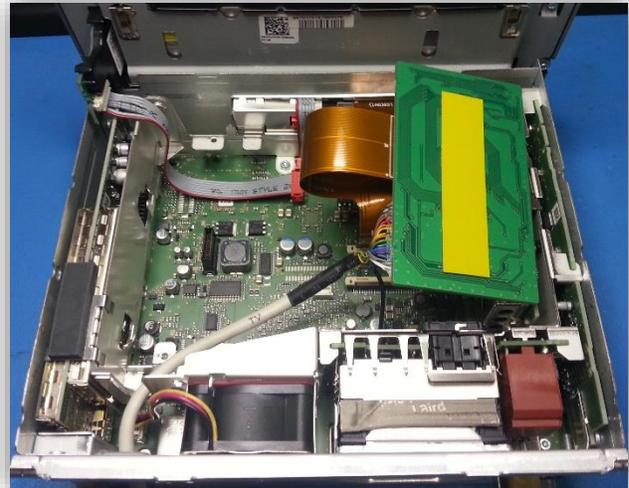
15. Use a tie-wrap (leave some slack) to secure the **LVDS Cable** to the chassis of the radio as shown, to prevent damage to the modification.
