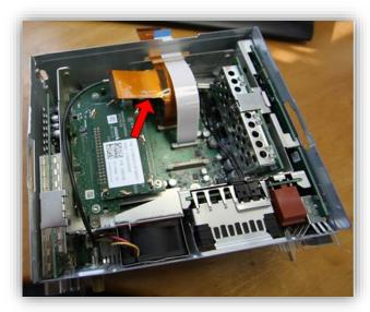
10. With tin-snips, cut a notch on the back side of the PCM chassis to run the LVDS cable through.
