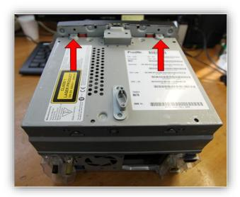
3. On the back of the radio, remove 3 torx screws.
