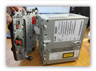
6. Slide the top half of the radio chassis towards the **rear**. It may be easier after you remove white QC sticker on the left side.
