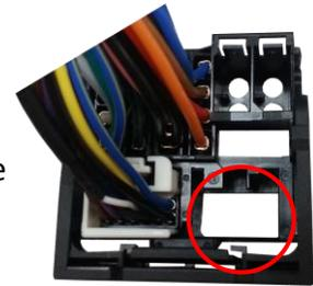
7. Connect the last free fiber optic pair back into the provided **fiber connector**. Connect this fiber connector to the port on the **SIR-PCM3** interface labeled 'MOST' (remove dust cover first).
