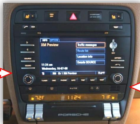
3. Remove (4x) Torx t20 screws that secure the radio into the sub-dash. Remove radio, disconnect all plugs and set the radio aside.
