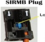
Use a pick tool to press the blue lock down from the side illustrated above and remove lock.
