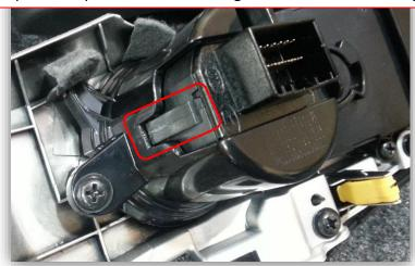
5. Remove (2x) Phillips head screws securing the radio:
