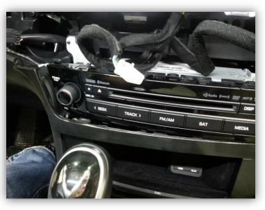
7. Remove (2x) Phillips screws that secure the lower dash pocket:
