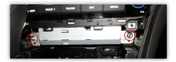
10. Pull the radio out of the dash, remove all connectors and set the radio aside.
