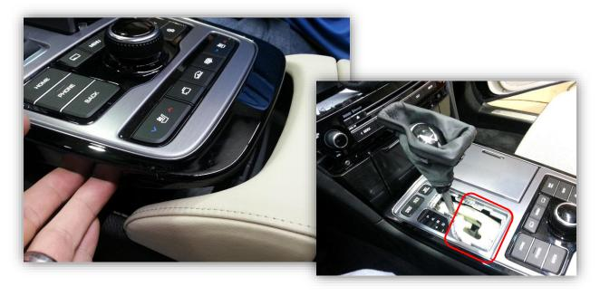
3. Remove the dash panel starting at the passenger side, pry carefully with panel tools. This panel can be removed as one piece with the cluster surround, or the cluster surround could be removed first. Note: the cluster surround connects to the top half of the steering wheel shroud.
