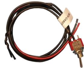
4. The **Pink wire** (input 3, pin 4) is used for **Palette Preset 2 Scrolling**. When this wire receives 12v (+) signal **through the provided momentary switch**, the FLIR camera will scroll through all available colors.\*
