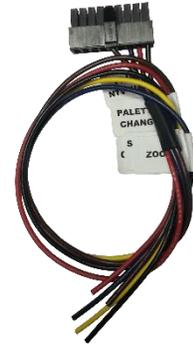
2. The **Red wire** (input 1, pin 2) is used for 2x zoom. When you provide this wire with 12v (+), the camera will zoom in. This wire is commonly connected to a high-beam (+) trigger so it will activate whenever high beam headlights are active.
