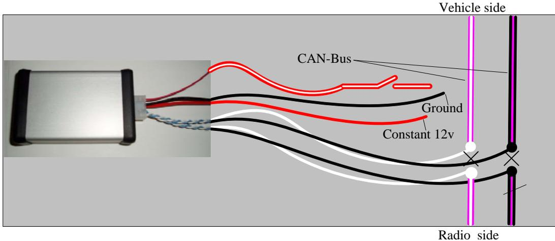
All wire connections **must** be soldered. The **red w/white** wire must be connected to 12 volts through a toggle switch. This toggle switch will activate video in motion. Please note: If the toggle switch is in the "on" position, navigation may not be functioning to it's full capacity until the toggle switch is back in the "off" position.
