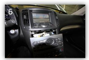
Gently pull the top section back and away from the dash to release the top clips. Make sure that the vehicle is off and disconnect all the harnesses from the back of the HVAC panel. DO NOT turn the key or push the push to start button until after the HVAC panel has been plugged back in during later steps.
