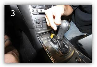
Insert the pick tool or a small screwdriver into the shift lock hole and depress the shift lock mechanism
