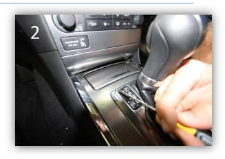
With a pick tool, remove the shift lock hole cover.
