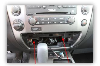
Remove the two screws at the bottom left and right with a phillips screwdriver. Above and at a 45 degree angle behind these two screws are 2 more screws. You must use a long phillips screwdriver to access them. Remove these screws as well.
