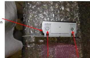
Mount the included touch screen monitor into the bracket, making sure that the angle side is facing the mark, secure it with the factory screws and reinstall the monitor back into the vehicle.
