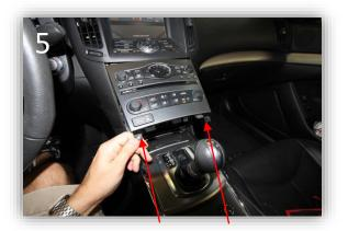
Remove the screws from the left and right bottom corners and pull the HVAC panel from the bottom up and away from the dash.
