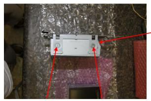
Mark the bracket on the side where the monitor has an angle. Remove and retain the 2 screws on each side of the factory monitor and remove it from the bracket. Beveled corner of touchscreen is the bottom
