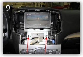
Remove the two screws holding the top of the radio bracket and the bottom of the monitor brackets.
