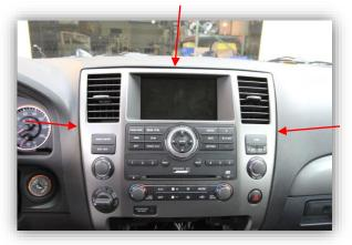
Using a soft pry tool, pry around the outside of the HVAC fascia to release the clips all the way around. Pull the entire fascia towards the back of the vehicle to release the clips, disconnect all the wiring harnesses and set aside.
