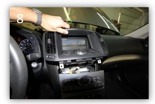
Pull the monitor shroud up and back towards the rear of the vehicle and remove it. The ribbon cable attached to the shroud should have already been removed in step 6.
