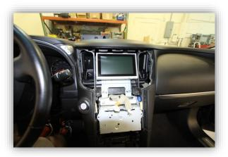
Remove the screws around the monitor bracket, unplug the monitor and set the monitor and bracket aside.
