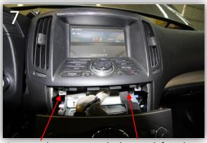
Remove the screws on the bottom left and right that holds the monitor trim in place. These screws were hidden by the HVAC panel.
