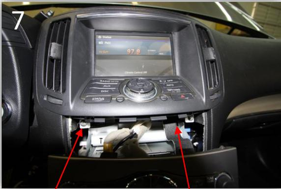
Remove the screws on the bottom left and right that holds the monitor trim in place. These screws were hidden by the HVAC panel.
