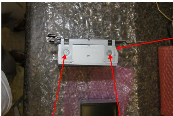
Mark the bracket on the side where the monitor has an angle. Remove and retain the 2 screws on each side of the factory monitor and remove it from the bracket.
