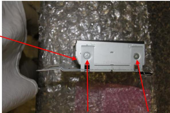
Mount the included touch screen monitor into the bracket, making sure that the angle side is facing the mark, secure it with the factory screws and reinstall the monitor back into the vehicle.
