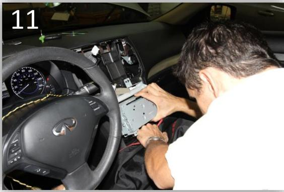
Pull the radio out of the dash, disconnect all wiring and set aside.
