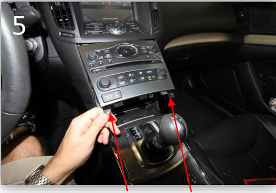
Remove the screws from the left and right bottom corners and pull the HVAC panel from the bottom up and away from the dash.
