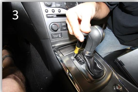
Insert the pick tool or a small screwdriver into the shift lock hole and depress the shift lock mechanism
