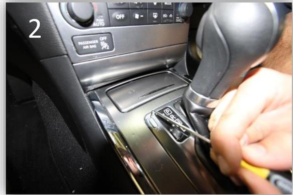
With a pick tool, remove the shift lock hole cover.
