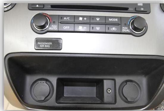
Using a soft pry tool remove the cover below the HVAC panel by prying gently around it to dislodge it from the retaining clips. Disconnect all plugs and set it aside.
