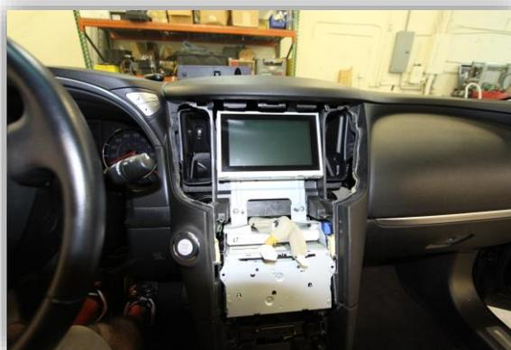
Remove the screws around the monitor bracket, unplug the monitor and set the monitor and bracket aside.
