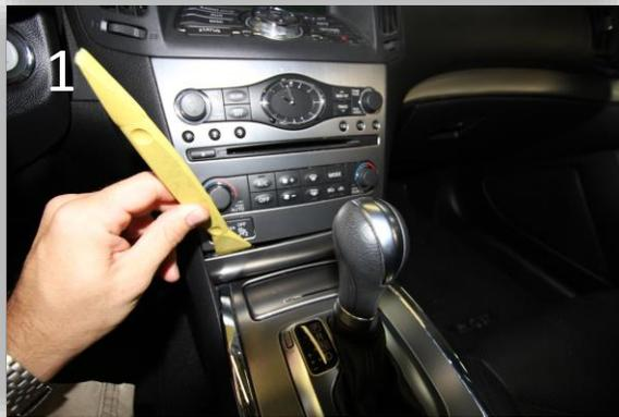
Remove the plastic trim ring around the shifter using a plastic pry tool.
