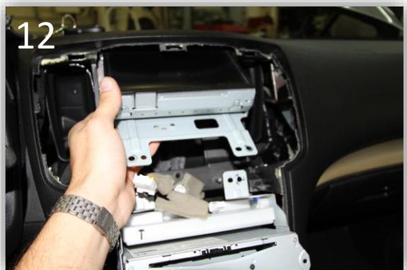
Swing the bottom of the monitor upwards to release the top of the monitor brackets from their U shaped top mount. Note: There are no top bolts and only a locking mount. Disconnect the monitor and set it aside.
