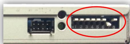
**\*Note: after adjusting Dip Switches, you must disconnect and reconnect power to the interface or the change will not be implemented.**
