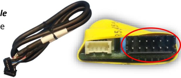
10. Connect the factory LVDS Video cable to the green LVDS port on the provided **SUB-Board**:
