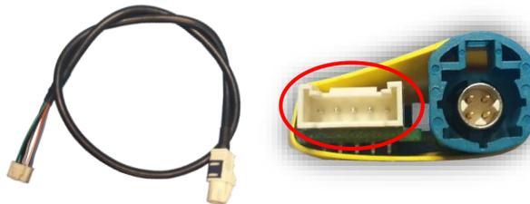
12. Connect the AV Input cable to the port on the W204 interface labeled '**AV IN/OUT**'. If you're only connecting a reverse camera (and no other inputs), the signal input from the camera must connect to the RCA labeled '**REAR-C**'. Refer to the dip-switch settings chart to skip/enable AV sources upon toggle switch presses (optional. Page 2).
