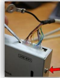
3. Connect the **AV Input** cable to the port on the CDR31 interface labeled '**AV IN/OUT**'. If you're only connecting a reverse camera (and no other inputs), the signal input from the camera must connect to the RCA labeled '**R-CAM**'. Refer to the dip-switch settings chart to skip/enable AV sources upon toggle switch presses (optional. Page 2).
