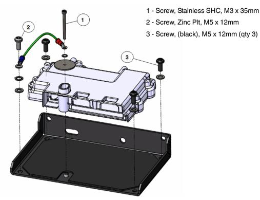
As shown in the drawing, a single stainless steel socket head cap screw secures a green grounding wire and the ECU to the ECU bracket. A single zinc plated pan head screw secures the other end of the grounding wire to the chassis.
