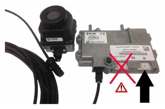
Connect the Power/Video Cable to the ECU connector designated with the Power indication, as indicated with the black arrow in the image.Do NOT connect the Video/Power cable to the connector indicated with a red X.
