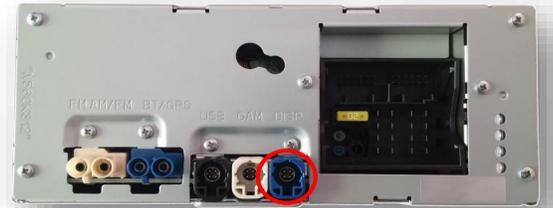
6. Connect the provided **Cam input harness** to the 4-pin port on the W205-RVC interface labeled '**CAMERA IN**'.
