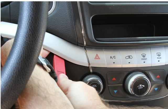
2. With the plastic pry tool, remove the plastic trim on the driver's side.
