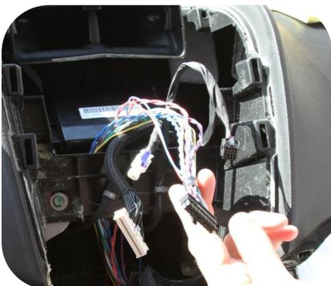
11. With the dash disassembled, route the end of the supplied T-harness to behind the screen location.
