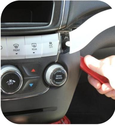
4. Using the plastic pry tool, gently pry the control panel from the dash.
