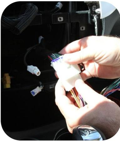
8. Take the 22 pin radio power harness and insert it into the female end of the supplied T-harness. (Forcing the connectors together may bend or push out pins in the harness. Take care when connecting).
