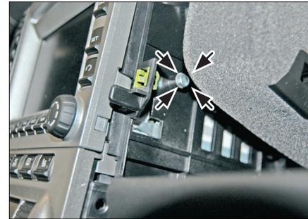
4. Loosen one screw (7 mm,) located at the right side of the head unit.
