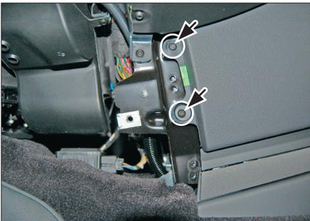
2. Remove 4 Torx (TX15) screws (2 on each side.)
