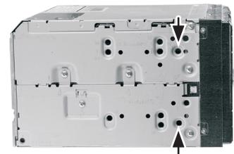
Mount the metal brackets to the Double-DIN head unit.
