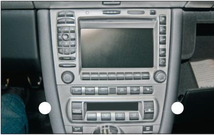
1. Remove 2 Torx (TX25) screws (1 on each side) left and right, located at the front end of the center dash.
