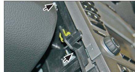
5. Release the 4 retaining brackets of the OEM head unit (2 on each side) by turning them 90° (see arrows)
