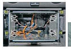
8. Use a soldering iron to heat up the plastic surface under the metal hooks left and right (4 on
