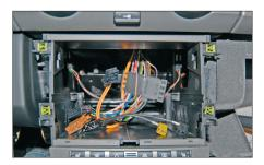
4. Loose one screw (7 mm,) located at the right side of the head unit.
