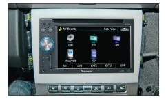
9. Push the head unit into the fixed metal frame until it snaps in.
