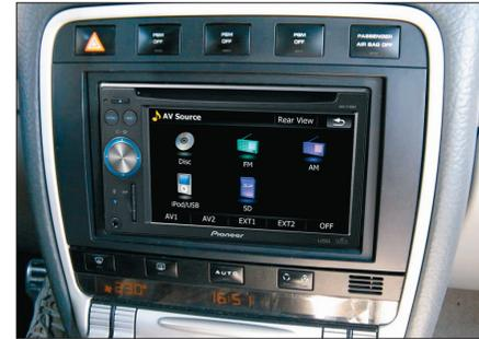
3. Place fascia plate on the dashboard. Fix it with the 4 original screws.
