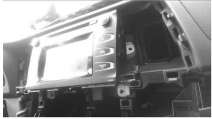
Remove (4) 10 mm bolts from radio bracket
