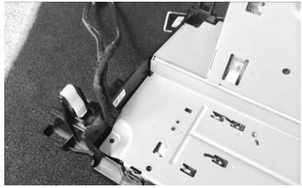
2in1 cable should exit the radio as shown. There is a small gap for it. Be carefully not to interfere with the screw hole as it might damage the cable when put screw back in.
