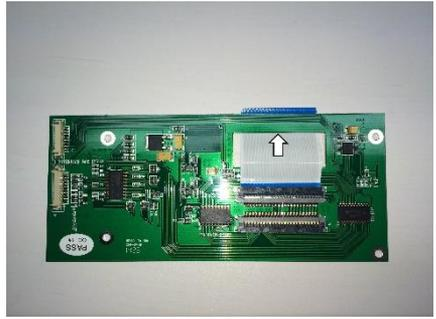
Prepare the ribbon cable to route under the opening
