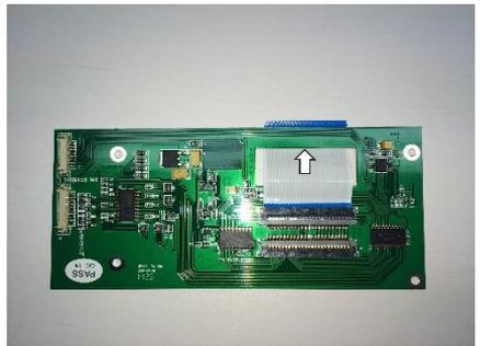
Prepare the ribbon cable to route under the opening
