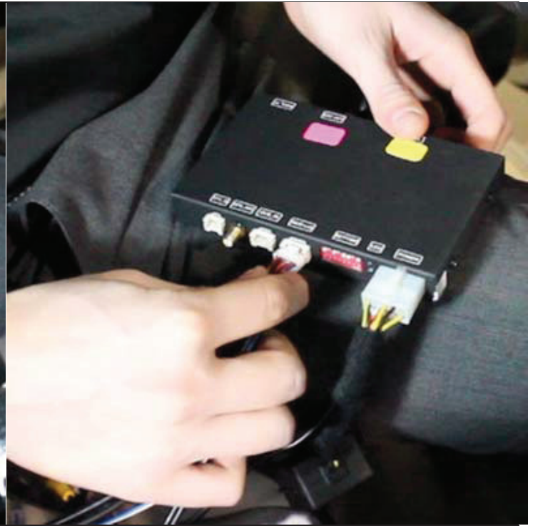
Connect the speaker interface harness to the navigation control module.
