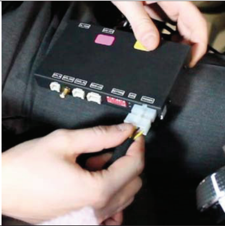
Connect the power harness from the vehicle interface harness to the navigation control module.
