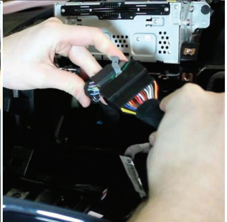
Connect the vehicle interface harness to the factory wiring harness on the car. ( Note: the large factory harness includes a locking retainer clip.)
