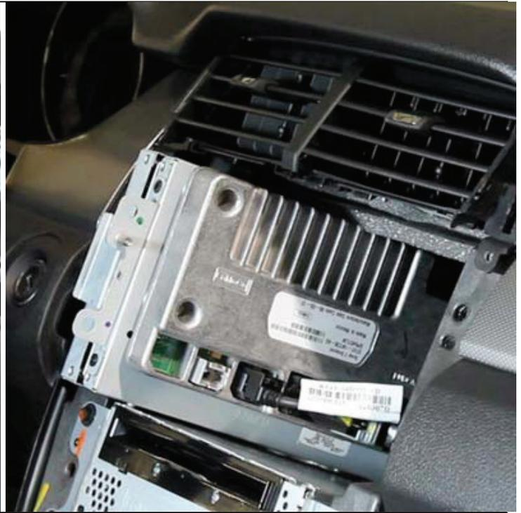
Gently turn the touch screen unit towards the driver's side of the vehicle to easily access the factory wiring harnesses.
