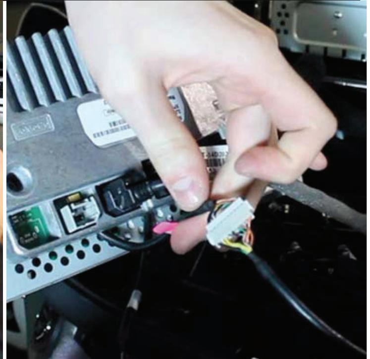
Attach the vehicle interface harness to the backside of the touch screen unit.
