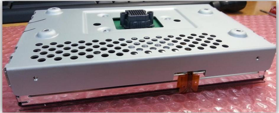
7. Now separate the metal housing from the LCD panel. Lifting the opposite side of the touch panel ribbon will give you easy access to remove the ribbon connectors:
