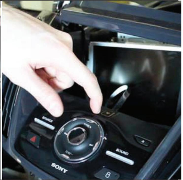
Replace the touch screen unit. Make sure no wires are pinched in the process.
