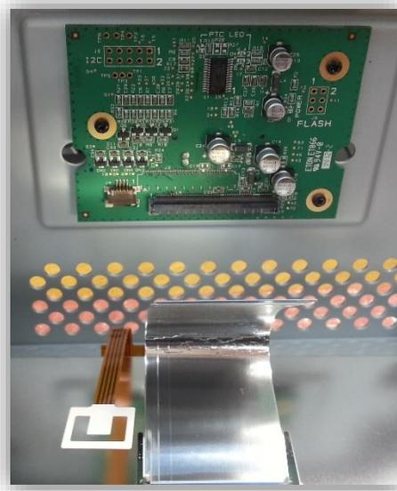
9. Lay the back metal housing down with the circuit board facing up in the orientation shown, and remove (3x) Phillips head screws:
