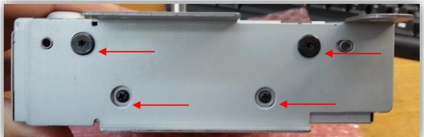
5. Next, remove (2x) Phillips head screws on the top and bottom of the LCD housing:
