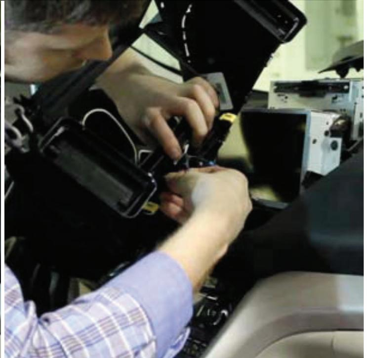
Remove the dashboard trim surrounding the touch screen unit using an automotive trim tool.
