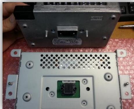
3. On the LCD panel housing, mark across the brackets and the housing to make replacing later a breeze:
