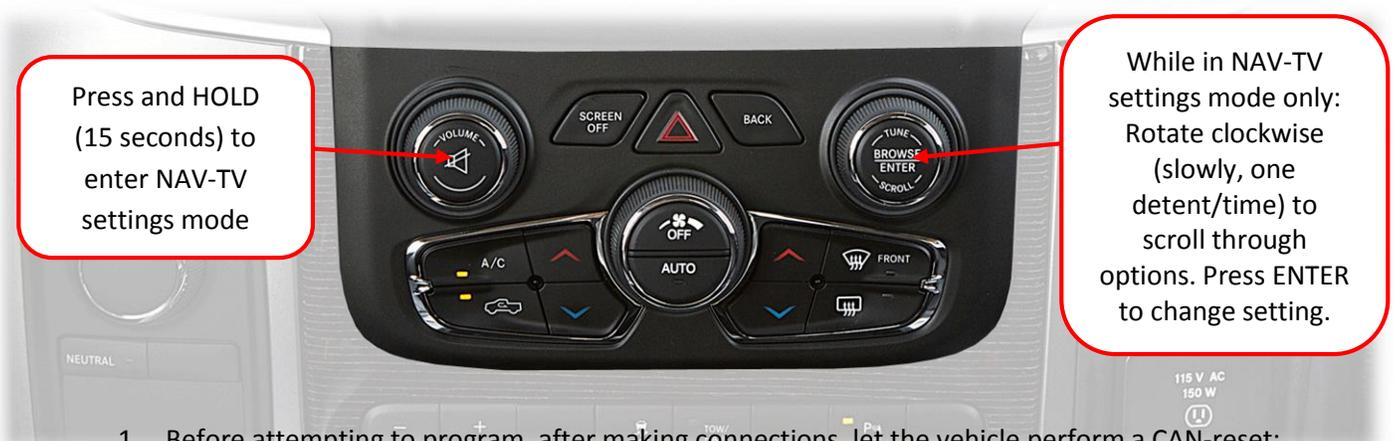
1. Before attempting to program, after making connections, let the vehicle perform a CAN-reset: Close all doors/trunk/hood, lock the vehicle and waiting 5 minutes before proceeding to program.
