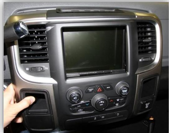
4. Remove (4x) 7mm screws that secure the LCD touchscreen.
