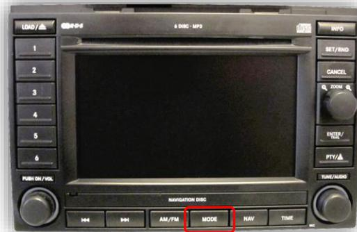
**Reverse Cam/Forced Cam:** Double press the main power button on the radio. This will automatically display the backup camera regardless of gear or motion of the vehicle. To return to the factory screen, double press the main radio power button again.
