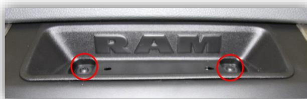
3. The face should be free now, pull straight outwards (towards you) with medium force. Use plastic panel tools if necessary.
