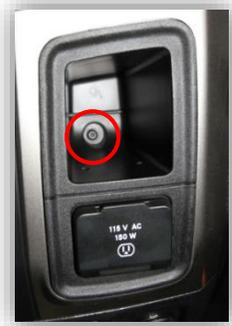
2. Remove (2x) Torx t20 at the top of the dash. They are hidden beneath a rubber mat.
