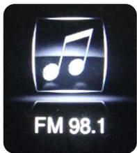
To show the FM source on the **cluster**, first clear any messages shown (door status, etc) with the UP or DOWN arrows on the steering wheel. Press the audio source button until 'FM' is displayed.
