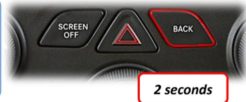
**Force Front Camera:** To force front camera, press and hold radio '**SCREEN OFF**' button for 2 seconds (truck chassis) or '**FRONT DEFROST**' (car chassis). To exit AUX mode, press and release the '**BACK**' button.
