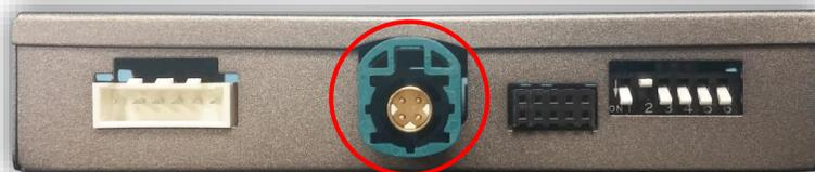
**NOTE:** If there is no dark blue LVDS video plug present, use the cable that makes the OEM screen disappear when unplugged (while radio is on).
