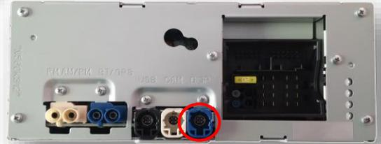
10. Connect the small white 4-pin plug labeled 'CAN2' to the plug on the W205-N interface labeled 'CAN2' for proper operation.
