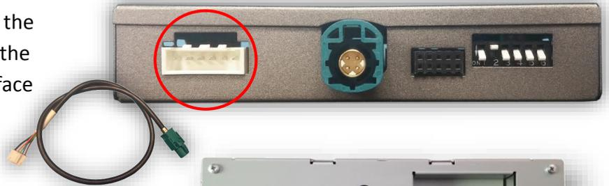
9. Connect the free end (aqua) of the provided **LVDS Video Cable** back to the factory radio at the 'DISP' (dark blue) port.
