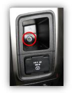
2. Remove (2x) Torx t20 at the top of the dash. They are hidden beneath a rubber mat.
