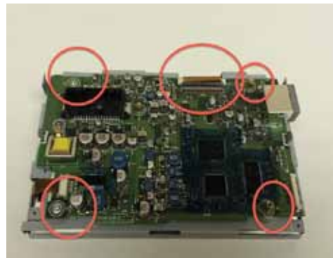
Remove Video Board screw and 2 ribbon cable
