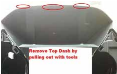
Remove top panel (pulling out with tools)
