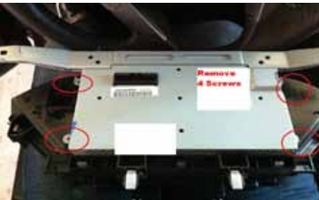
Remove 4 screws Take out LCD Panel
