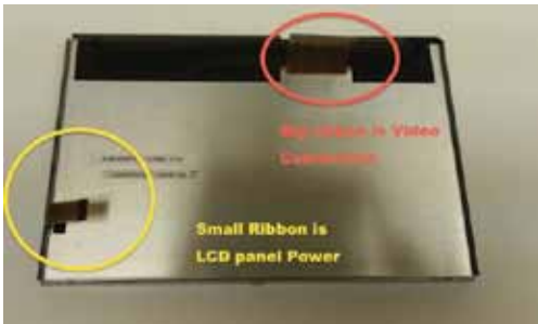
unscrew factory video board and get ready to take off LCD panel
