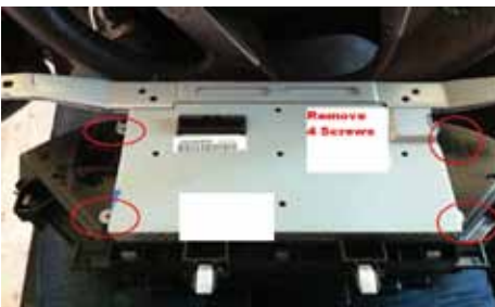
Remove 4 screws Take out LCD Panel
