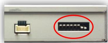
**\*Note: If the dip switches are not configured prior to installation you must remove power to the unit prior to making adjustments to the dip switches. When power is reconnected after the dip switch adjustment the new settings will be stored into memory.**
