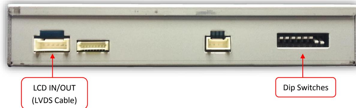
Dip Switch Settings\* Configure prior to installation
