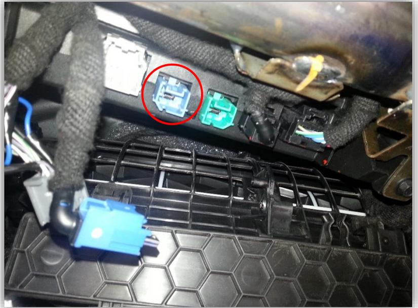
4. Plug the factory **blue** mini-USB connector into the black, female end of the provided LVDS cable.
