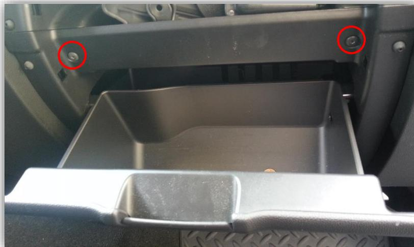
2. GM trucks only: Underneath the glove box you'll find (2x) more additional Torx T15 screws firing upwards. Remove these and pull the glove box free from the dash (all that remain are clips).
