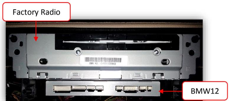
*For double-din radio stacks, you'll need to find another mounting location. Dropping the passenger glove box may be necessary.*
