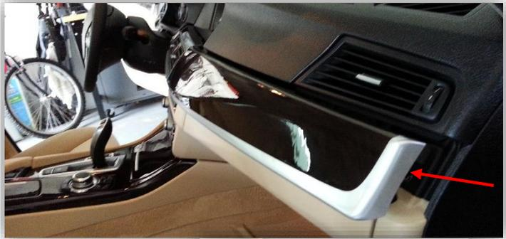
2. Disconnect all harness connected to this panel (near the vents mostly). You may want to remove the push button ignition switch so that you can test the BMW12 interface prior to replacing the dash panels. Either unclip this assembly or remove (3x) Torx screws and then reconnect to the vehicle plug:
