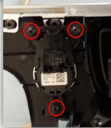
3. Remove (2x) Torx screws securing the radio controls and climate control face, pry outwards and disconnect all harnesses:
