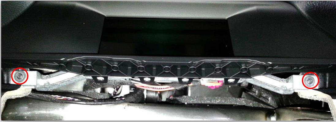
2. Remove the factory monitor and disconnect the circular LVDS video cable. Reconnect the free end of this **(factory) LVDS cable to the BMW12 interface at the port labeled 'LCD-IN'**.
