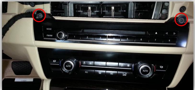
4. You should now see the disc-player portion of the radio. Remove this assembly by removing (2x) more Torx screws:
