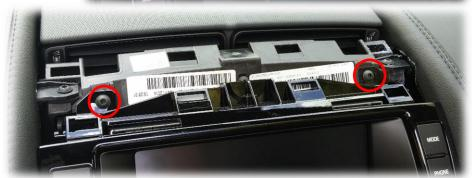
6. Using a plastic tool and hook tool, carefully pull the trim surrounding the climate knobs towards you. This panel must be pulled straight forwards.
