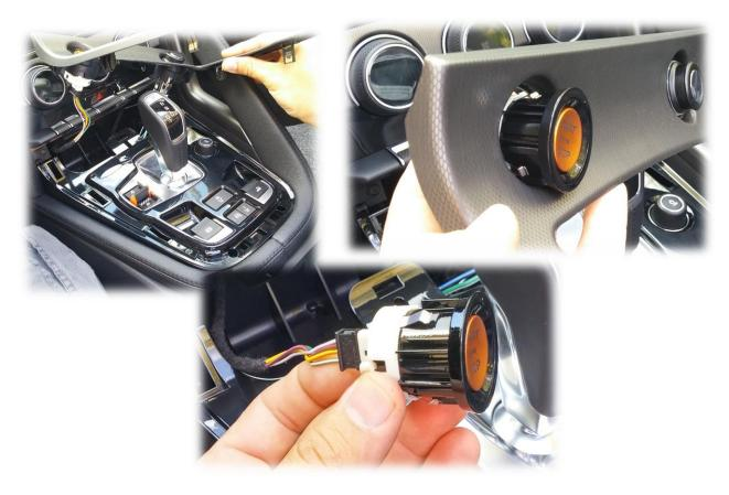
3. Remove (2x) Torx t20 screws securing the bottom half of the climate control.
