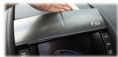
5. Remove (2x) Torx t20 screws securing the screen bezel:
