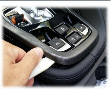
2. Disconnect the cigarette lighter plug and the push button ignition switch plug. It helps to remove the push button ignition switch and reconnect it to the plug (for testing).
