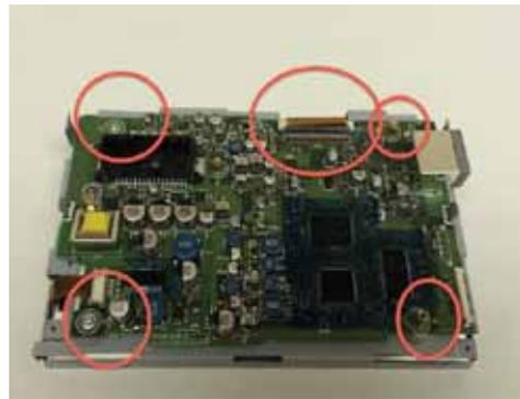
Remove Video Board screw and 2 ribbon cable
