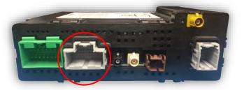
Connect the provided *Power/GMLAN T-Harness* in between the radio and the factory gray 20-pin harness.
