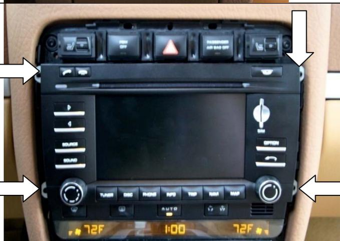
2. Remove (4) t20 torx screws from the sides of the radio and pull the radio gently out of the dash in order to disconnect all stock cables and antenna connectors.
