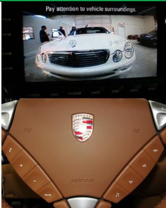
1. Place the vehicle in reverse and your image will appear on the screen. When putting the vehicle back in drive the image will stay on the screen for up to 20 seconds or until the vehicle reaches 7 mph.
