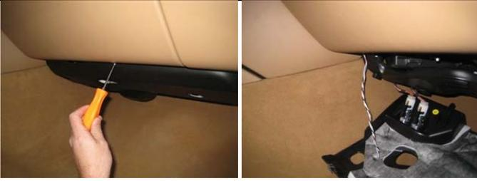
5. Drop the plastic panel over the passenger side kick panel area by taking out (1) t20 Torx screw and pulling the panel towards the floor. Run the black, white/blue and white/red wires from the new radio harness into the opening as in the picture to your left. These wires will power your reverse and front cameras, as well as the video switcher.
