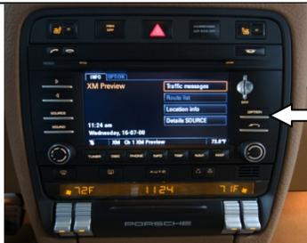
3. After the radio reboots first select the option button on the right of the PCM. Then select "rear view camera" and then make sure the "automatic" feature is highlighted. Automatic means that every time the vehicle goes into reverse the PCM screen will show the backup camera image.
