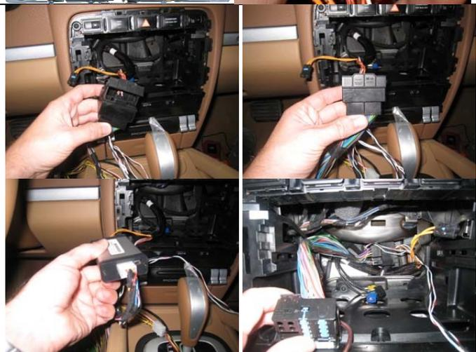
4. With the fiber unplugged from the factory harness plug the aftermarket harness into the original harness and secure it by closing the stock locking tab. Attach the PCM3CAM module to the aftermarket harness and secure the filter to the back of the radio cavity with either double sided tape or Velcro. Fold the harness in the cavity as shown to allow clearance for the radio.
