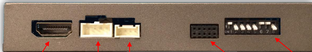
HDMI Cable from HD-LINK Not Used Expansion Board Control Not Used Dip Switches
