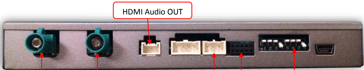
Video OUT (to screen) Video IN (from radio) HDMI Audio OUT IR Eye Not Used Dip Switches
