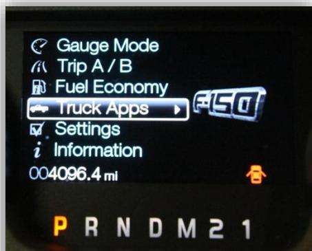
1. Using the steering wheel controls scroll down to the **Truck Apps** function in the instrument cluster.
