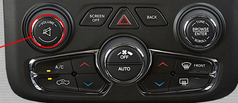
**Force Rear Camera:** To force rear camera, press and hold radio 'BACK' button for 2 seconds. To exit forced rear camera, press and release radio 'BACK' button. **Note: this function is NOT supported on vehicles equipped with a factory reverse camera.**
