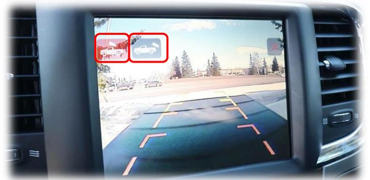
*\*NOTE: whenever Cargo or RVC is activated through this menu system, the vehicle's speed is ignored so the camera will remain until deactivated. This may affect the OEM navigation (while active only).*
