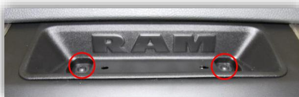
3. The face should be free now, pull straight outwards (towards you) with medium force. Use plastic panel tools if necessary.
