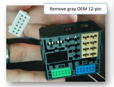
Connect OEM 12-pin to provided 12-pin (black, PIN-side). *NOTE: printed arrow location on provided 12-pin plug vs OEM plug.*
