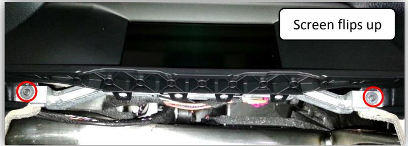
2. To access the iDrive harness, remove the panel surrounding it (may have Torx screw securing to sub dash)
