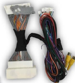
4. Connect the 4-PIN ***'PAD'*** plug among the T-Harness to the interfaces' ***'CAN'*** port if the vehicle has a touchpad-style controller.
