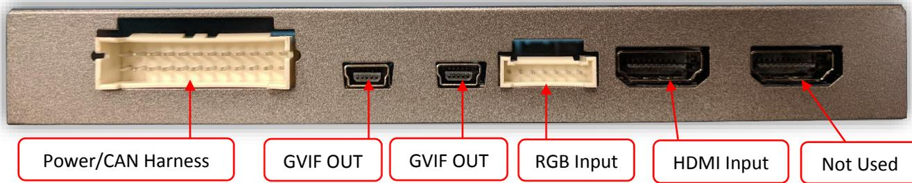
Power/CAN Harness      GVIF OUT      GVIF OUT      RGB Input      HDMI Input      Not Used
