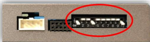
**Disconnect power before adjusting dip switches.**
