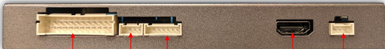
Power/CAN Harness      Expansion Board      RGB Input      HDMI Cable from HD-LINK (optional)      Not Used
