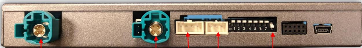
Video OUT (to screen)      Video IN (from radio)      Not Used      IR Eye      Dip Switches
